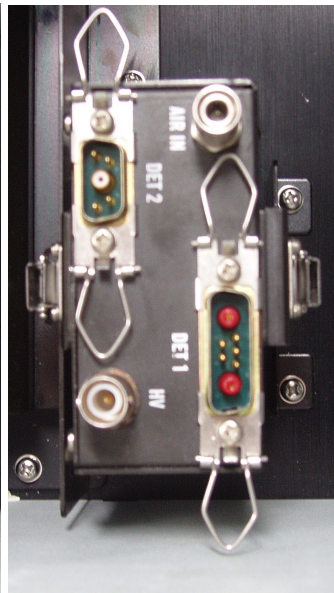
All cables and locks were removed from the detector.
