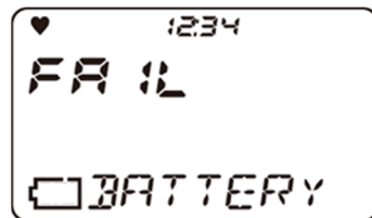
Battery voltage abnormality
