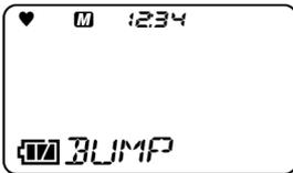
The LCD display shows a heart icon, a battery level indicator, and the number '1234' at the top. Below this, the word 'BUMP' is displayed in a large, stylized font.         | P. 43 |
